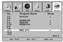
4 Press ▲ or ▼ to highlight the channel you want to delete, then press ENTER to mark the channel. A check mark disappears if the channel is deleted. The check mark appears if you add back the channel.
